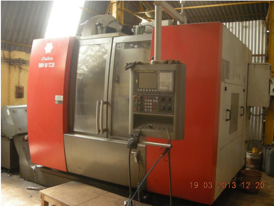
03) CNC VERTICAL MACHINING CENTRE, BFW MAKE: MACHINE SIZE: X-800 MM X Y-450 MM X Z-450 MM
