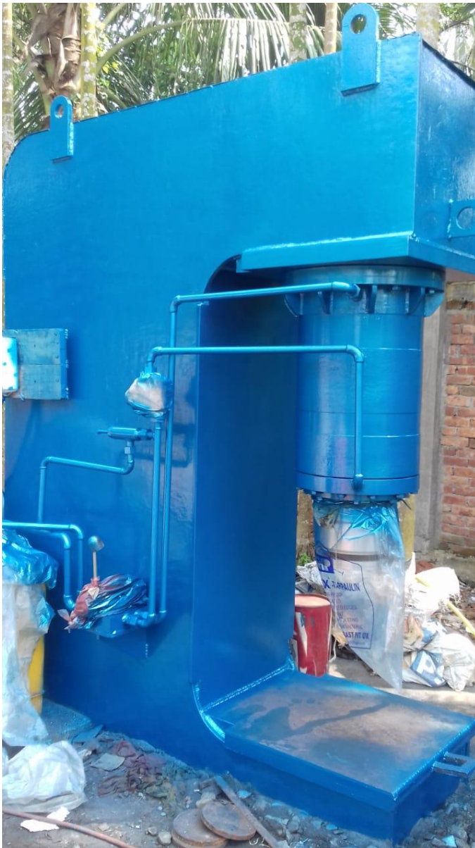
28) Bending Machine, 25 Thickness X 2000 mm Width Plate Bending Machine
