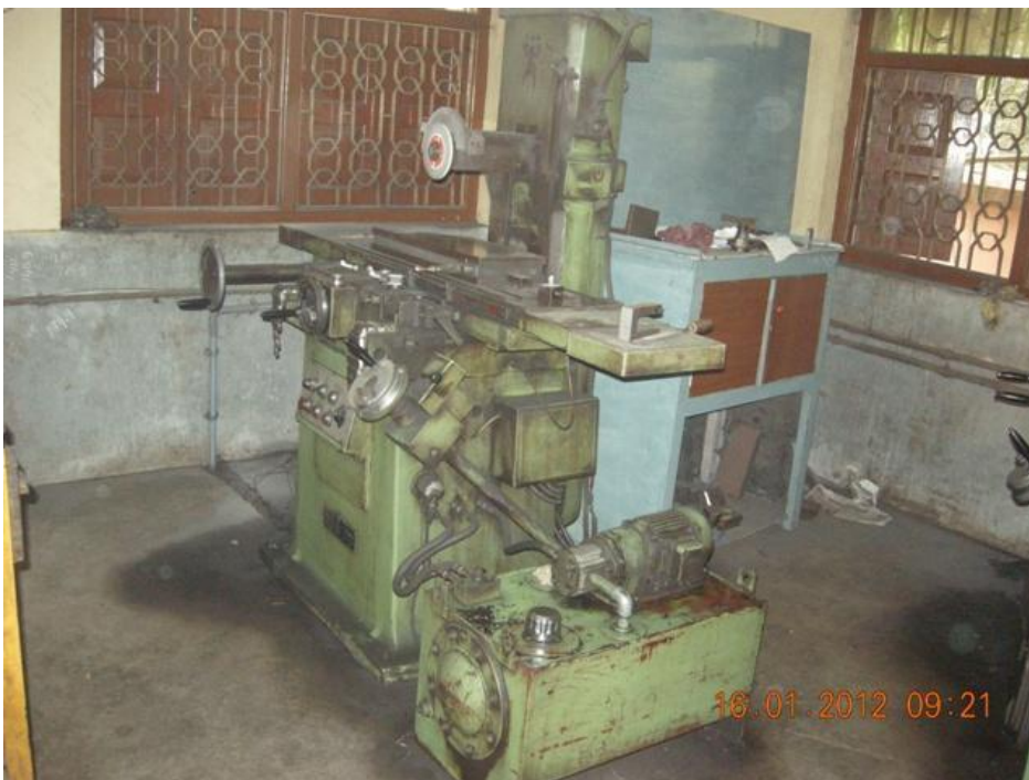
23) 80 SPINDLE Dia HORIZONTAL BORING MACHINE, MAKE-WMW, GERMANY
