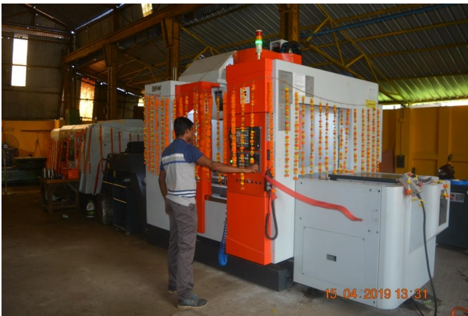
04) CNC TURNING CENTRE, BFW MAKE: CHUCK SIZE: 310 MM Ø X 700 MM LENGTH
