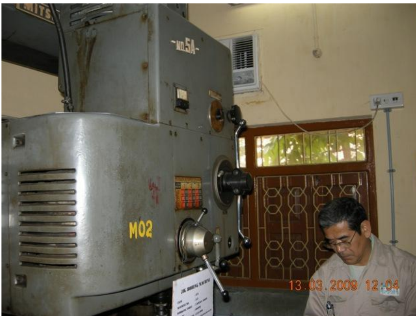
07) HORIZONTAL BORING MACHINE, MAKE:WMW, GERMANY
